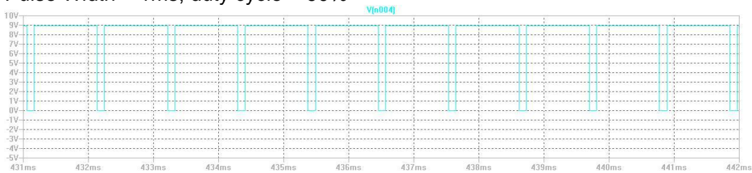
Figure 16 – By adjusting the value of resistor R2, various duty cycle can be obtained
