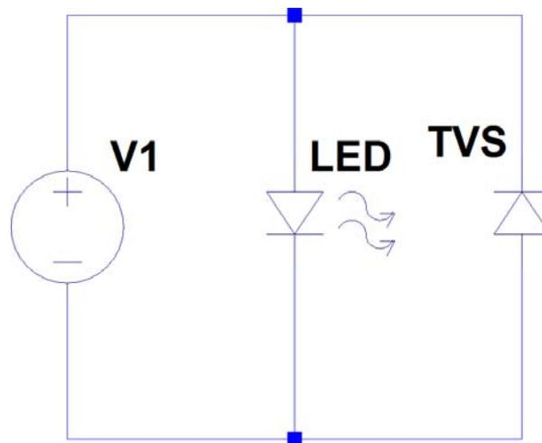
**Figure 1: Function of TVS diode**
