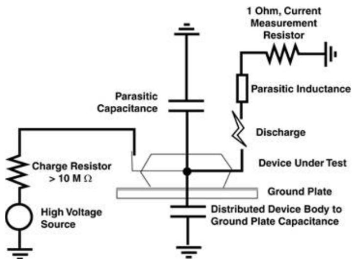
**Figure 4:** Typical CDM test
