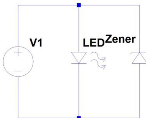
**Figure 5:** Reversed Zener diode connected in parallel with LED
