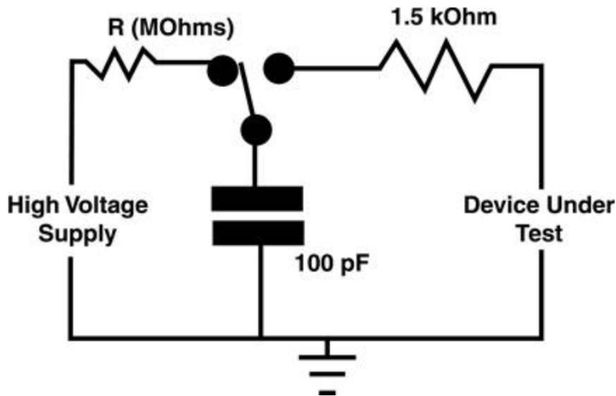
**Figure 3:** Typical HBM circuit
