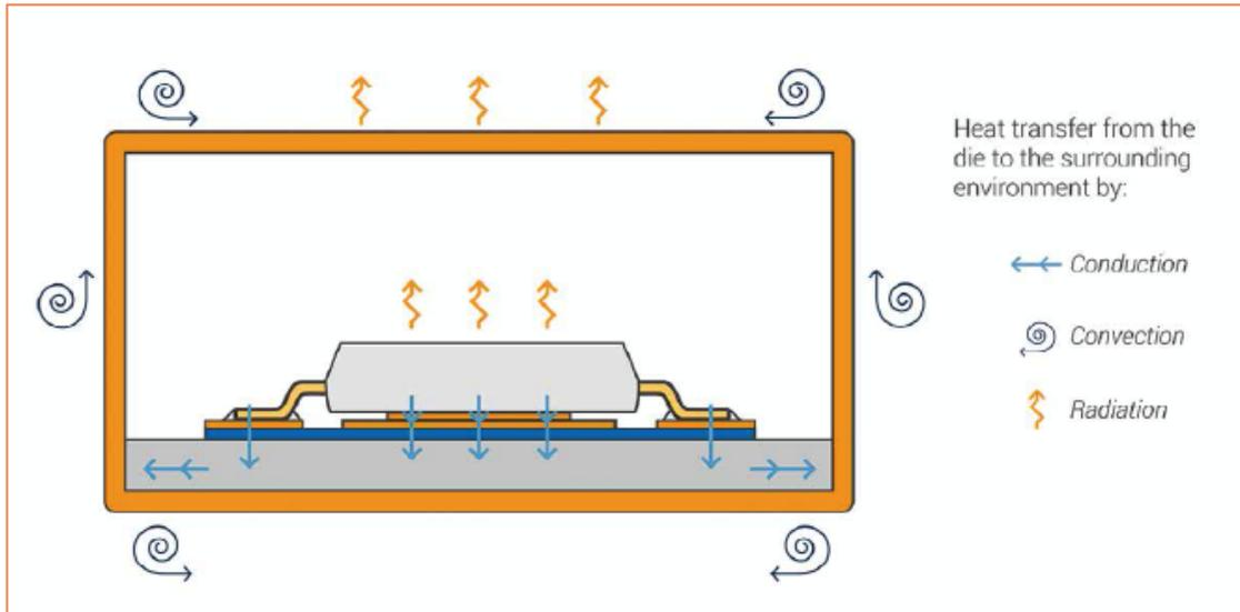
**Figure 6:** Heat transfer in LED system
