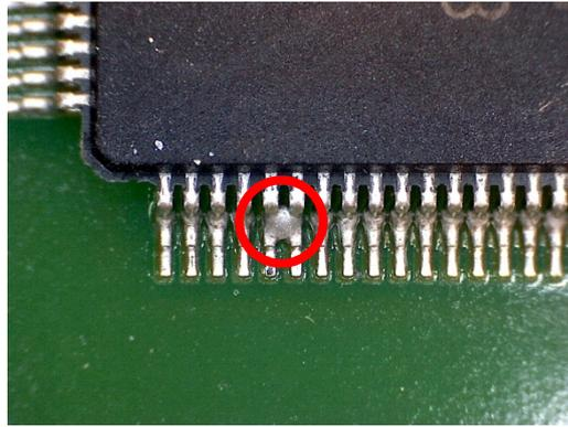
**Figure 7:** Example of solder bridging of an IC
