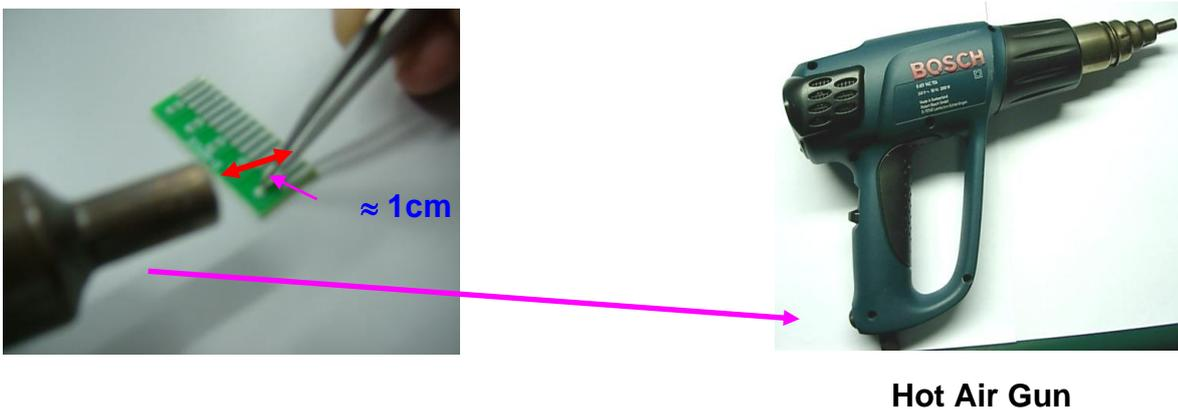
Use hot air gun set at 350°C to blow it at a distance of approximately 1cm. This will take about 15 to 20 seconds to disconnect the connections.
