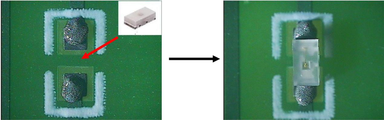
Finally use hot air gun set at 350°C to blow it at a distance of approximately 1cm. This will take about 15 to 20 seconds for the solder paste to melt and form the connections. Please refer to figure 3.
