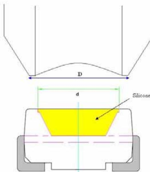
Figure 1: Pick & place nozzle diameter (D) should be larger than the opening (d)
