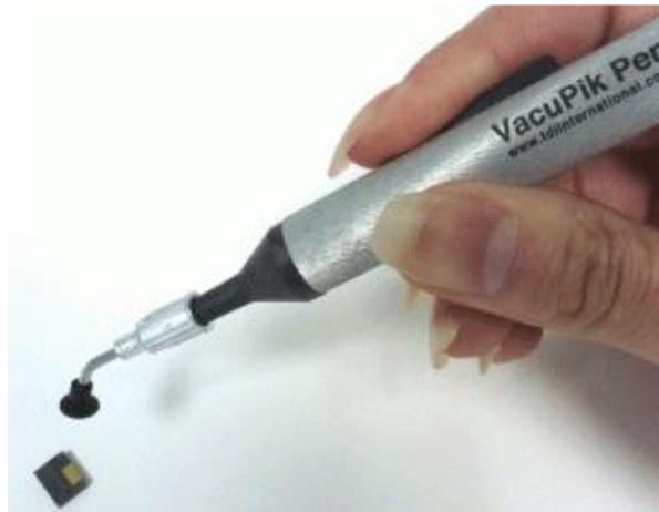
Figure 10: Example of vacuum suction pen
