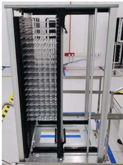
Figure 7: Example of carrier to store the PCB after SMT
