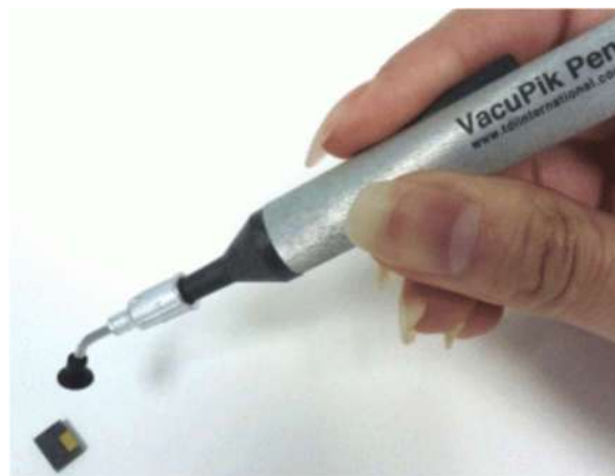
Figure 17: Example of vacuum suction pen
