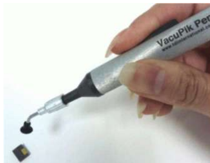
Figure 18: Example of vacuum suction pen
